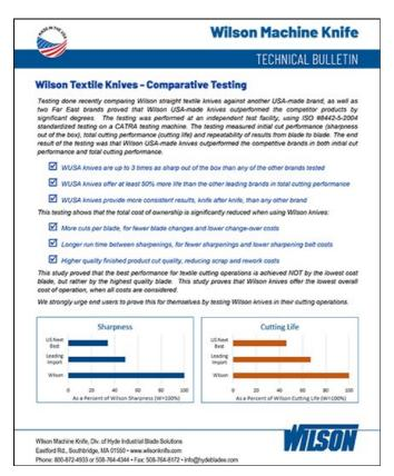
Performed at an independent test facility using ISO#8442-5-2004 standardized testing on a CATRA machine, Wilson USA-made Cloth & Textile knives outperformed competitive brands in both initial and total cutting performance. Testing measured sharpness out of the box, cutting life and consistency of quality and results from blade to blade. Download the full report:
